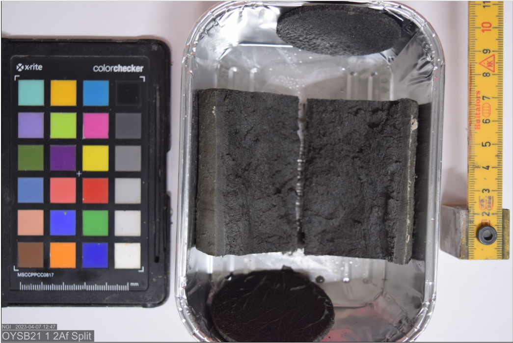
Figure 7.3: Split specimen 2Af after triaxial hydraulic conductivity test.
