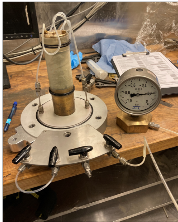
Figure 5.10: Installation of specimen 2Bf on triaxial base pedestal in walk-in freezer. Also showing applied vacuum -20 kPa.
