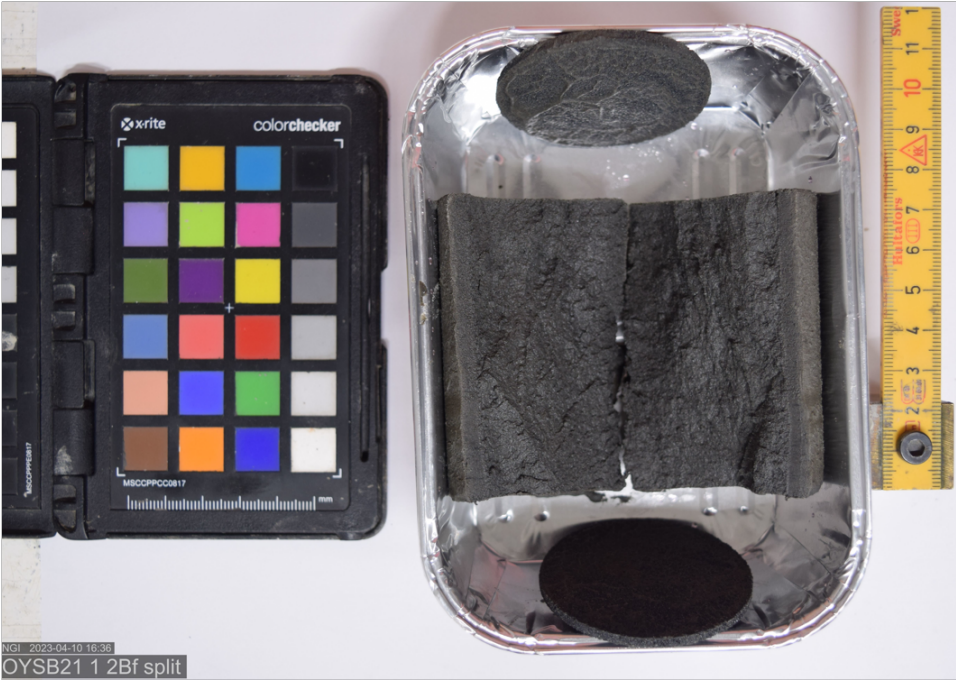
Figure 7.5: Split specimen 2Bf after triaxial hydraulic conductivity test.
