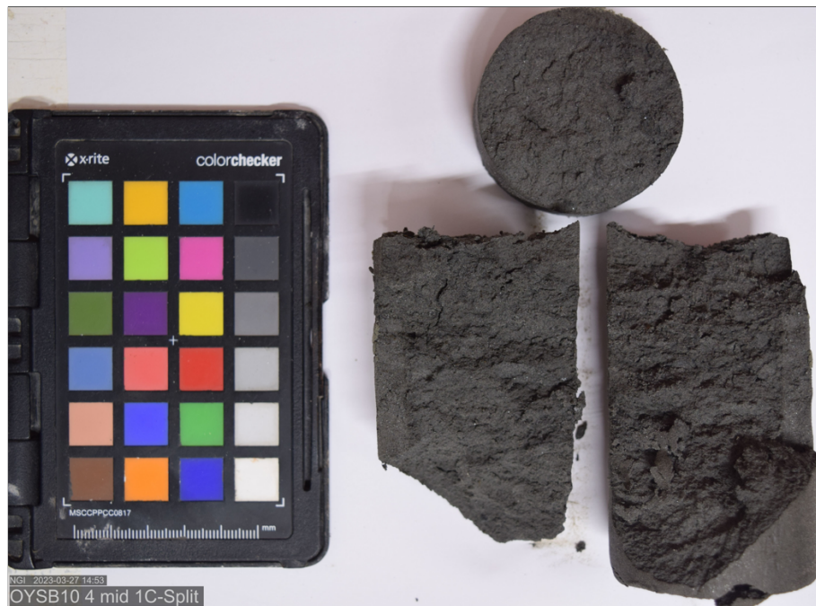
Figure 7.8: Split specimen 1C after triaxial hydraulic conductivity test.
