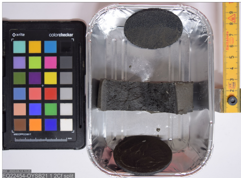
Figure 7.7: Split specimen 2Cf after triaxial hydraulic conductivity test.
