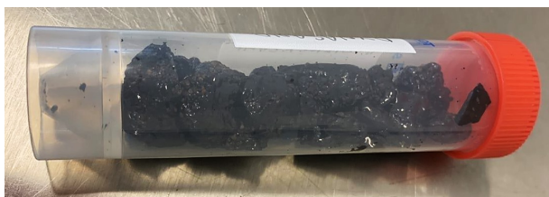
Figure 5.2: Picture of the condensed hydrocarbon residue from an anode baking furnace off-gas cleaning facility. From Arnesen et al.[70], with permission from Springer Nature.
