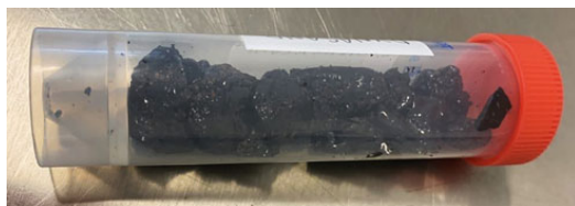
Fig. 1 Picture of the condensed hydrocarbon residue from an anode baking furnace off-gas cleaning facility
