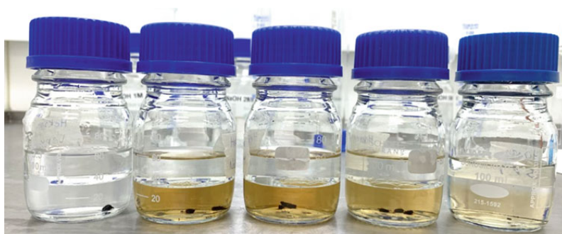
Fig. 2 A series with sample dissolved in n-hexane and increasing concentration of NaOH (left to right: Water, 1.0 M, 2.0 M, 3.0 M, and 5.0 M). Organic phase is on the top and aqueous is on the bottom of the flask
