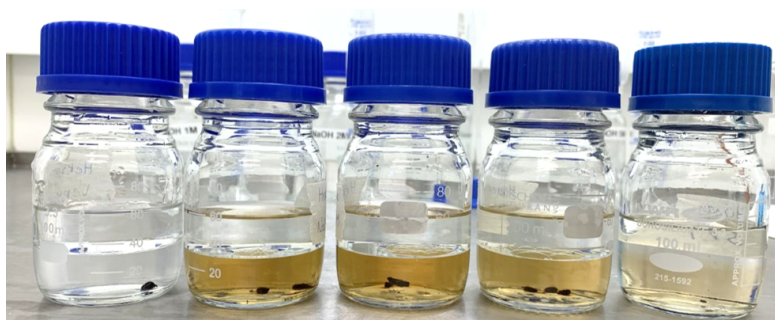
Figure 5.3: A series with sample dissolved in n-Hexane and increasing concentration of NaOH (l - r: Water, 1.0 M, 2.0 M, 3.0 M, 5.0 M). Organic phase is on the top and aqueous on the bottom of the flask.
