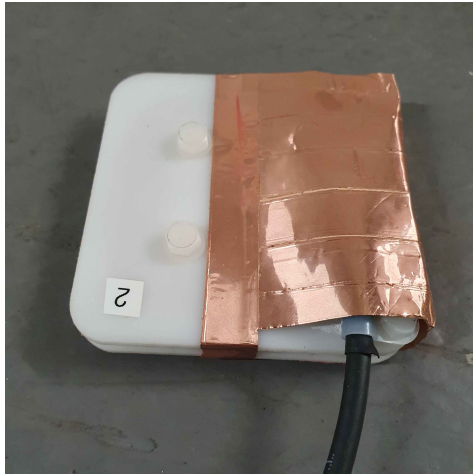
(a) The magnetic sensor used to measure the stray flux on the stator backside.
