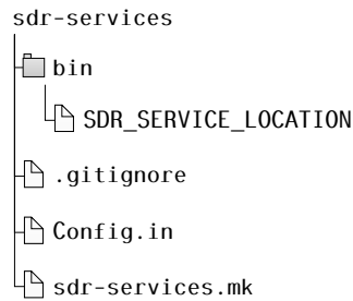
Figure 4.8: sdr-services dummy package. The sdr-services.mk file copies sdr-services and m6p-time-sync if they are present in bin/
