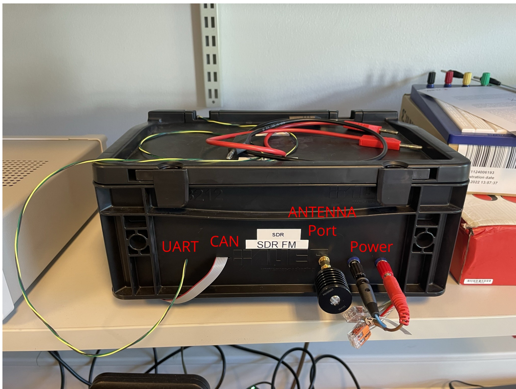
Figure 4.16: The finished safe environment for the FM version of the TOTEM. already connected to the HYPSON-2 LidSat.
