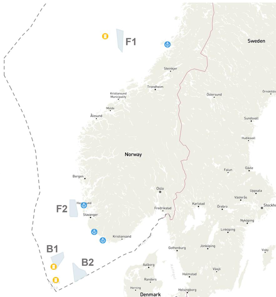
Figure 6.1: Map of hypothetical farms considered for simulation where F1 is Nordvest B, F2 is Utsira Nord, B1 is Sørvest B and B2 is Sørlige Nordsjø II
