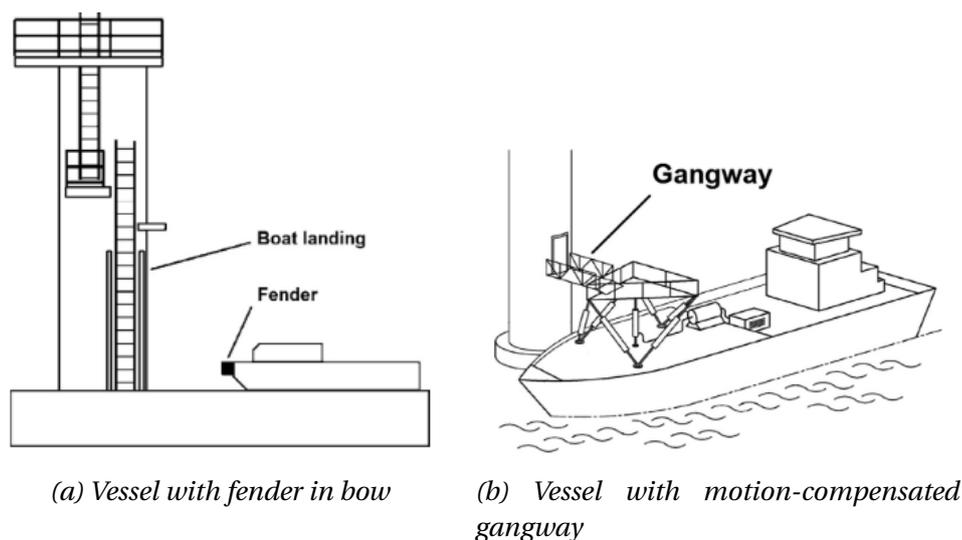
Figure 2.11: Docking options for transfer vessels (Guanche et al., 2016)
