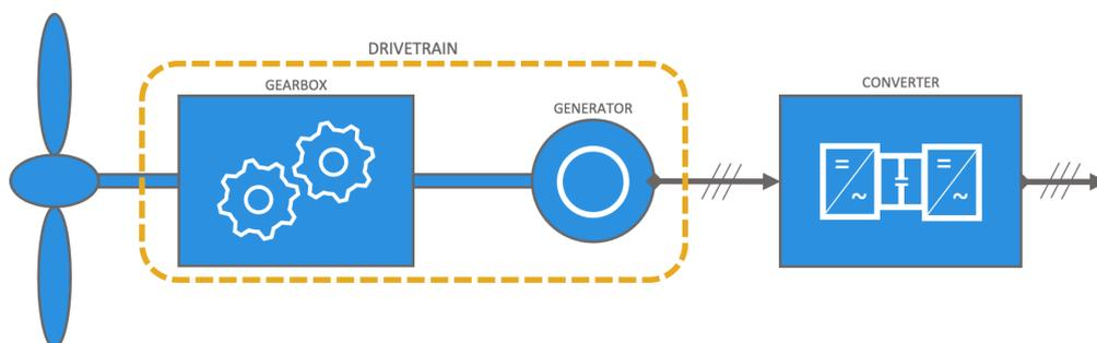
Figure 2.7: Schematic of a drivetrain with a gearbox interpreted from Nejad et al. (2022)
