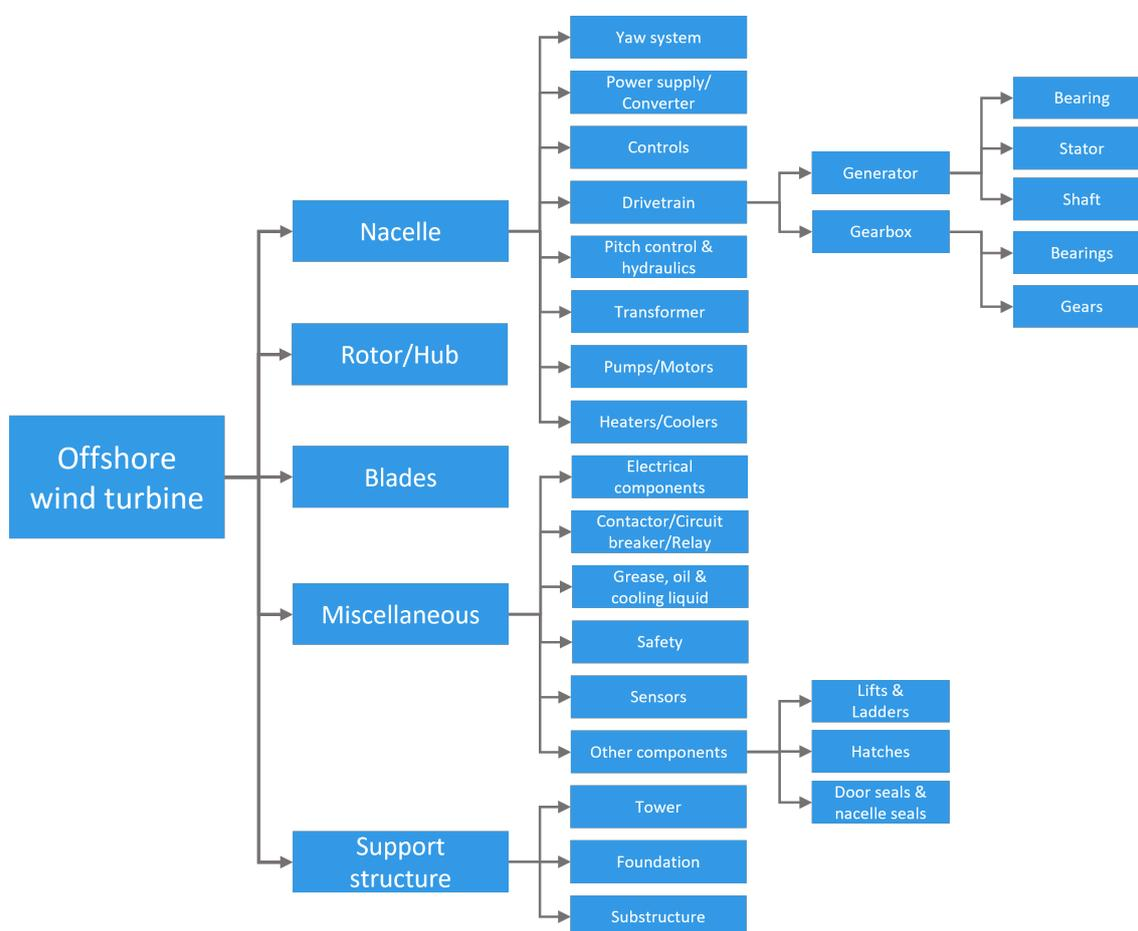
Figure 2.6: Breakdown of OWT's internal components
