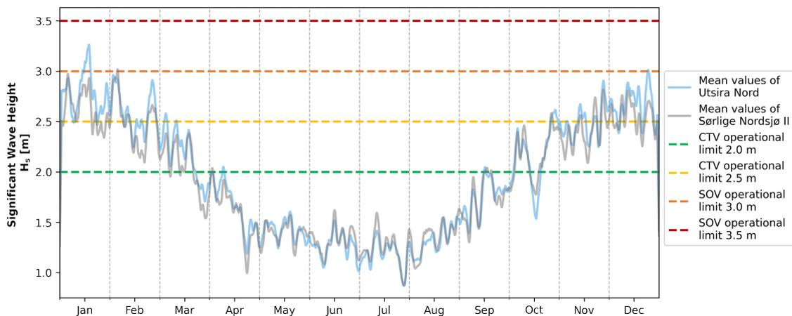
Figure 3.3: Mean wave heights (Appendix C) for Sørlige Nordsjø II and Utsira Nord compared to operational wave limits for vessels
