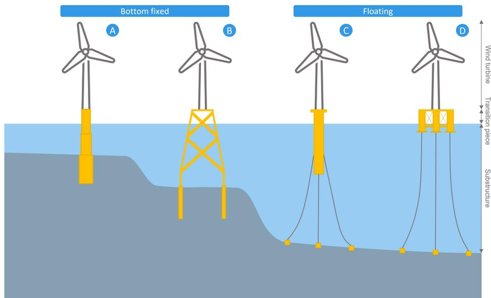
Figure 2.9: Illustration of substructures of OWTs
