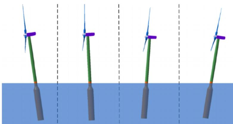
Figure 3.9: Pitching motion of a floating OWT (Tran & Kim, 2015)
