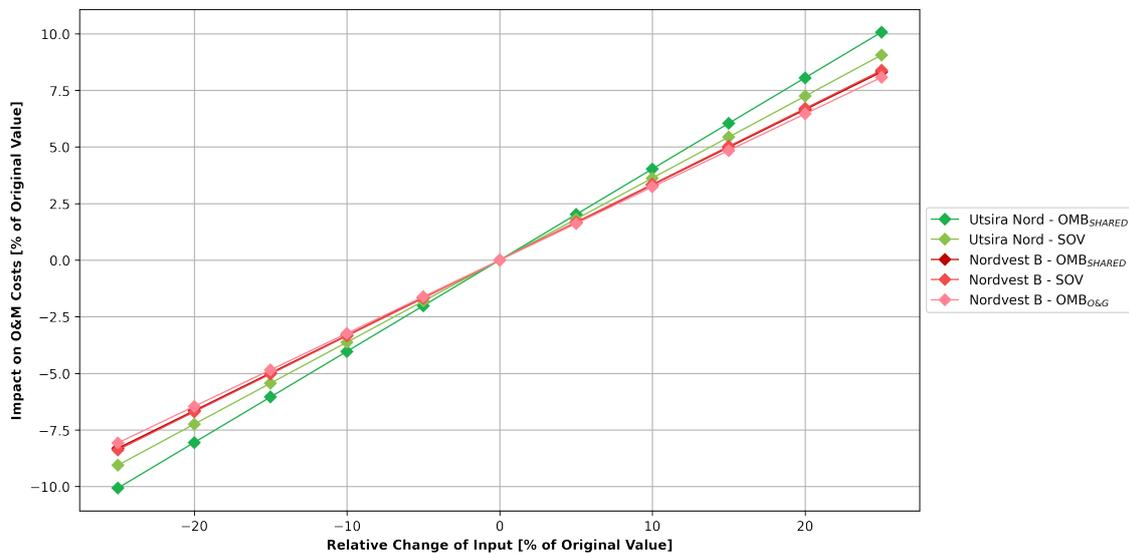
Figure 7.12: Sensitivity of the repair cost of the semi-submersible OWT
