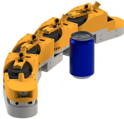
Figure 1.1: Illustration of the previous design of the Boa snake robot with five links. Figure retrieved from Löwer et al. [18].
