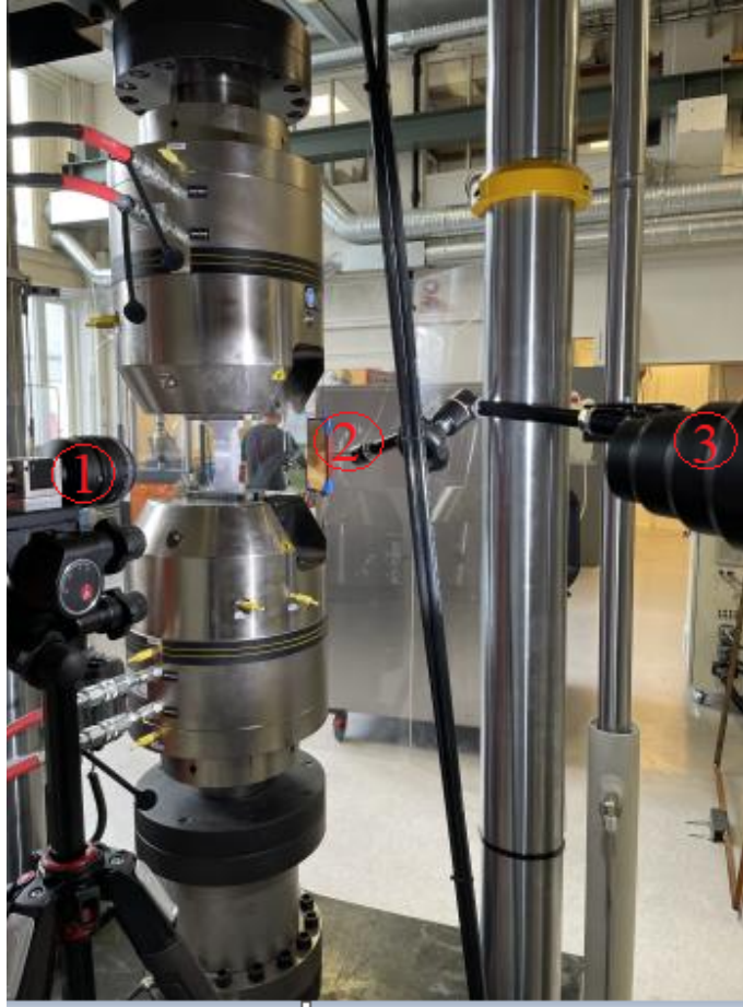
Figure 28: Test setup showing the camera (1), the mirror (2), and the light source (3).
