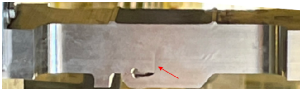
Figure 38: Image of 2Gap 16mm specimen under fatigue loading captured moments before fracture. Shows opening of the unbonded region and crack initiation at the bottom of the weld.
