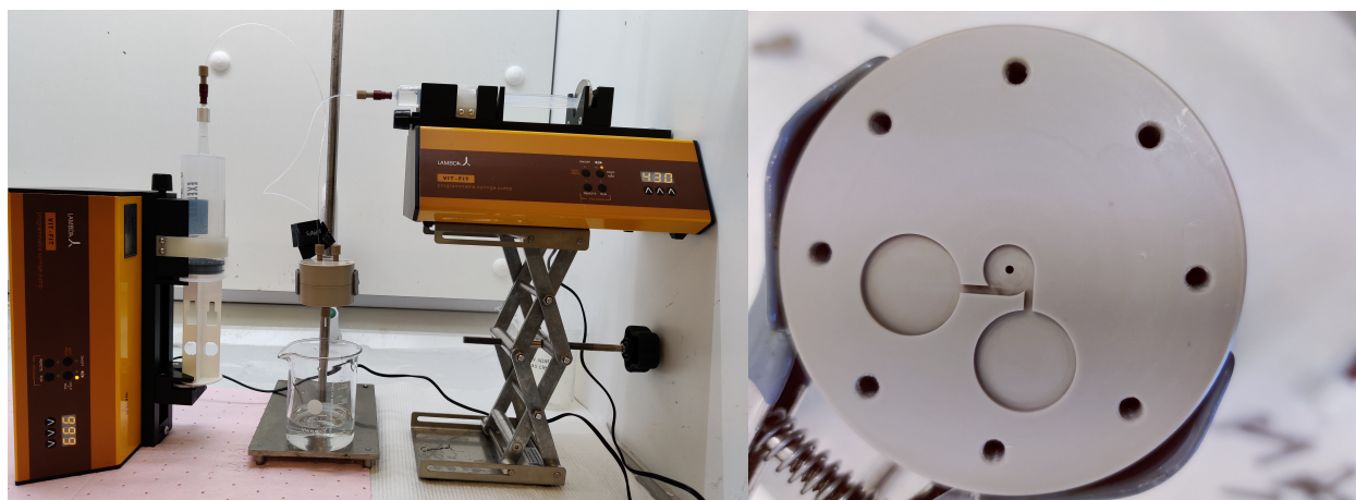
Figure 12: Inside view of MIVM (right) for FNP; FNP setup (left) with both syringe pumps for aqueous and organic phase.
