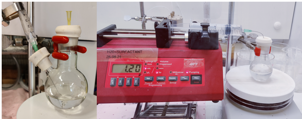
Figure 10: Nitrogen purging setup for PAA-OH/ PAA-PLGA and PEG-PCL (left); semi-batch addition of glycolide in THF to lactide, PEG and DBU dissolved in DCM.
