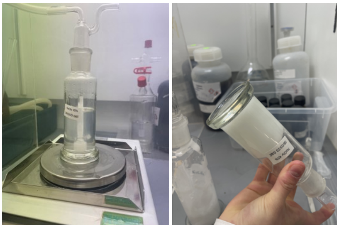
(a) 45wt% SG solution before the experiment (b) 45 wt% SG solution after 5 min of \text{CO}_2 injection
