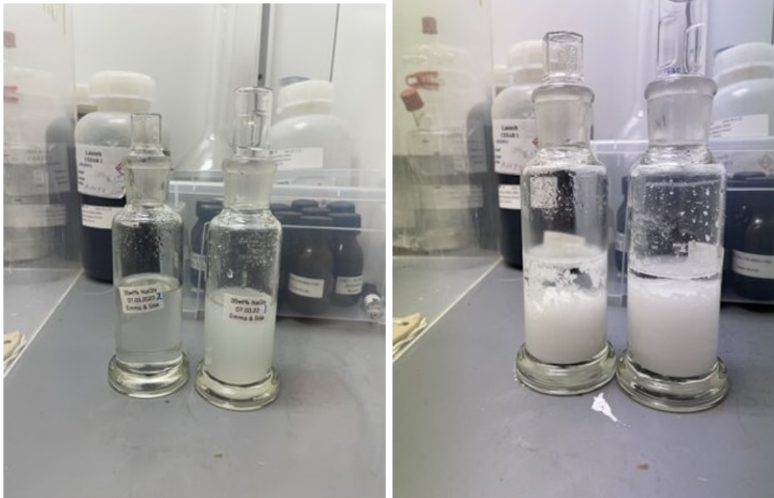
(a) 35 wt% SG solution, to left beaker just finished experiment and to right beaker 1 hour after experiment (b) 35 wt% SG solution 24 hours after experiment
