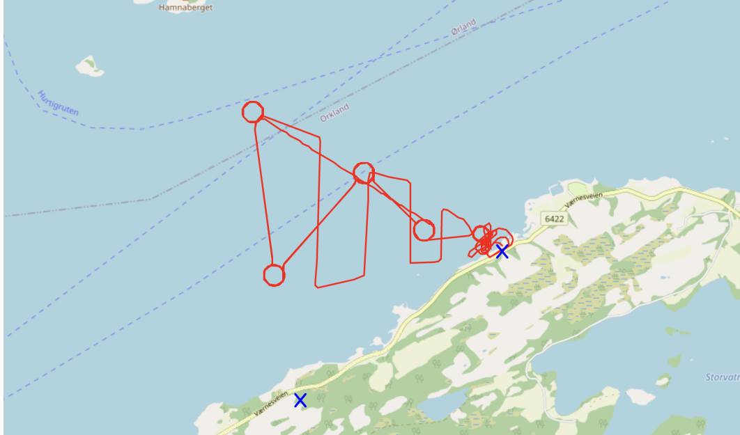
Figure 6.4: Flight path from Raustein, Agdenes over Trondheimsfjorden. The blue “x-es” correspond to the PARS locations. PARS 1 is located where the UAV starts and stops. PARS 2 is at the lower left side. Map data from OpenStreetMap. ©OpenStreetMap contributors [ODbL]
