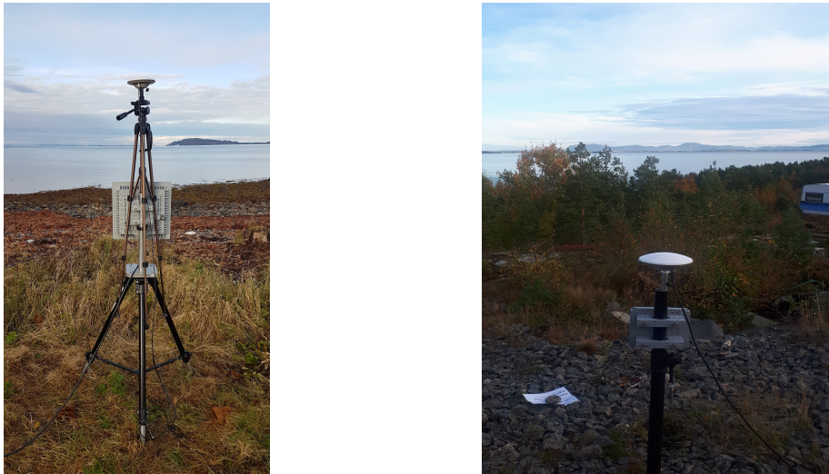
Figure 6.2: PARS 1 and 2 as well as RTK base stations mounted on top. Photo source: NTNU UAV Lab [55].
