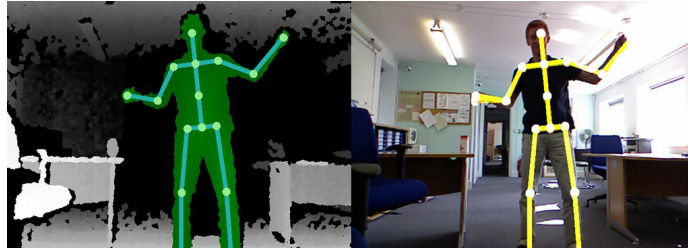
Figure 14.8: Kinect uses a depth-sensing and colour to register movement
