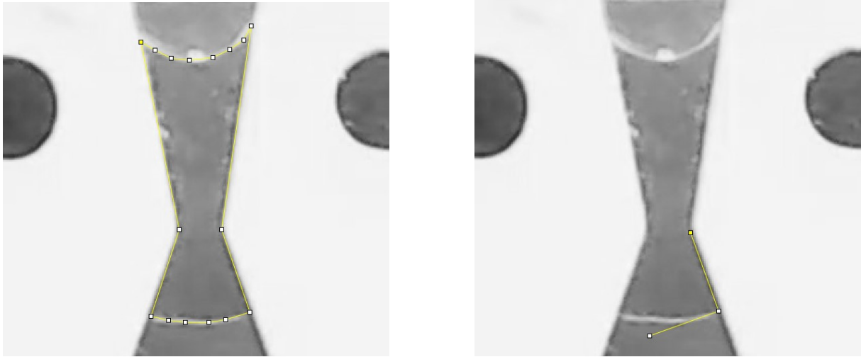
Figure 6.9: Examples on measuring a) the total volume of fluid, and b) the contact angles
