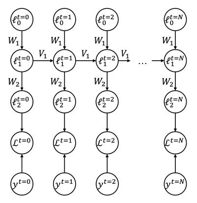
Figure 2.6: Unfolded recurrent neural network with a single hidden layer.
