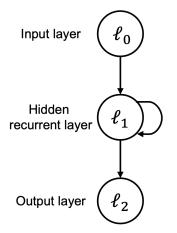
Figure 2.4: Example of a recurrent neural network with a single hidden, recurrent layer.
