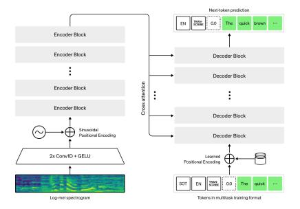
Figure 3.5: Whisper uses an off-the-shelf Transformer architecture with a slightly modified encoder. Since the model input is audio and not text, the audio needs to be converted to a log-mel spectrogram, which is then processed by the added convolutional layers with a GELU [21] activation function. The remaining architecture is identical to the original Transformer. (Source:<sup>1</sup>)
