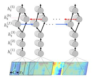
Figure 3.2: Deep Speech uses a relatively simple model architecture comprising four non-recurrent linear layers and a single bi-directional recurrent layer. The audio is converted to a spectrogram and fed to the model, which outputs a probability distribution over the English alphabet. (Source: [19])
