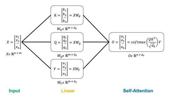
Figure 2.8: Self-Attention in a Transformer takes the input sequence  $\mathbf{X}$  and computes the key (K), query (Q), and value (V) matrices using a linear layer. Lastly, the output matrix O is obtained by computing a softmax using K and Q and computing the dot product with V. The matrix resulting from the softmax determines how much each value vector in V contributes to each output vector in O.
