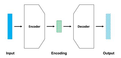
Figure 2.7: Dataflow of an autoencoder. The input is mapped to an encoding using the encoder, while the decoder takes the encoding as input in an attempt to reconstruct the input to the encoder.
