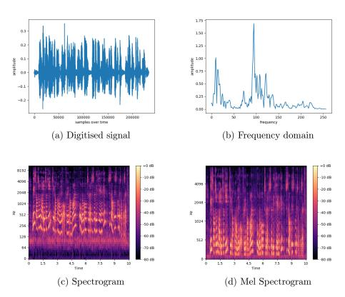
Figure 2.1: All figures are obtained from the same speech extract at the Norwegian parliament. The speech was obtained from the Norwegian Parliament Speech Corpus (NPSC) [35] dataset. (a) depicts the raw, digitised signal. (b) shows the time-frequency domain of a small window of the audio signal using 512 samples. (c) is the spectrogram resulting from the signal in (a) and (d) is the resulting spectrogram with frequencies mapped to the Mel scale.
