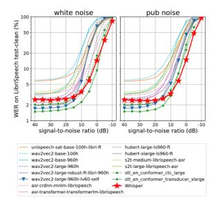
Figure 3.4: Noise performance of Whisper compared to other state-of-the-art speech recognition architectures when exposed to white noise (left) and real-world noise obtained from a crowded pub (right). The WER is based on the LibriSpeech [30] test-clean split. Whisper is outperformed by NVIDIA STT Conformer-CTC models from the NeMo toolkit [18], [25] under low noise conditions, but it scores a lower WER than other architectures for signal-to-noise ratios smaller than 10 dB. (Source: [31])
