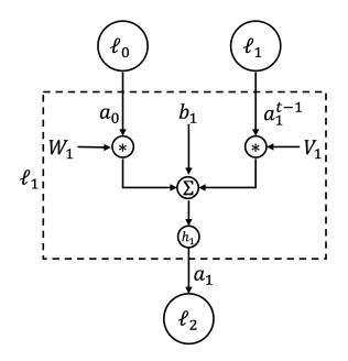
Figure 2.5: Visualisation of the computations performed in a hidden layer  $\ell_1$  with recurrent connections at time t. The activation from layer  $\ell_0$  and the activation  $a_1^{t-1}$  of layer  $\ell_1$  at time t-1 serve as the input to layer. The resulting output  $a_1$  is forwarded to the next layer. It also serves as the input to the recurrent layer  $\ell_1$  at time t+1 (not visualised).
