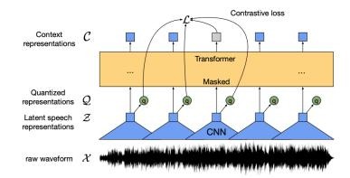
Figure 3.3: Wav2Vec 2.0 processes raw audio waveform data using a convolutional neural network to compute a latent representation  $\mathbf{Z}$ . The latent representation is then used to compute both a set of quantised representations and context representations. (Source: [4])
