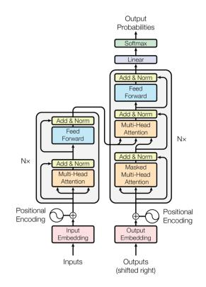
Figure 2.9: A Transformer comprises an encoder and a decoder, each consisting of a set of consequential, identical blocks. A single block in the encoder contains multi-head attention and a feed-forward layer. The decoder blocks use the same architecture, with the addition of a masked multi-head attention layer to prevent the model from attending parts of the input sequence that are beyond the current sequence position. (Source: [38])
