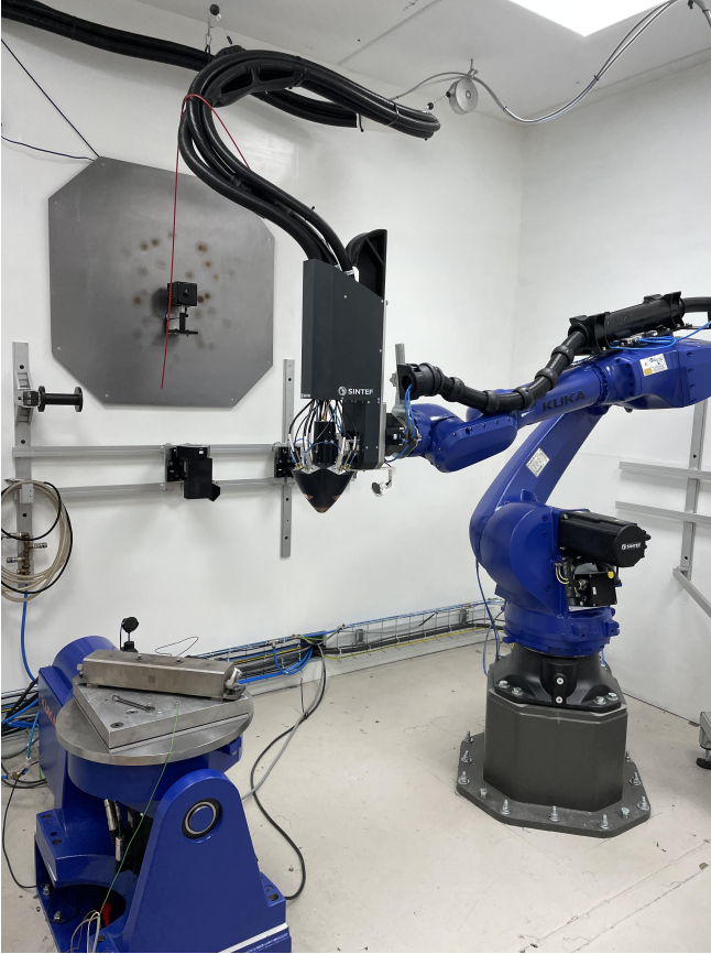
Fig. 1: The MELTIO system integrated with a KUKA Industrial robot for DED processes.
