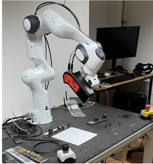
Figure 4.1: Illustration of the setup using Franka Emika robot arm and VC Nano 3D-Z.
