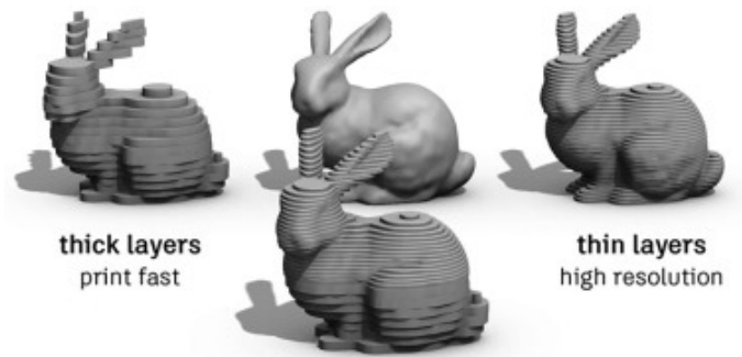
Figure 2.3: An example of slicing a solid geometry into horizontal layers with varying thicknesses. Thinner layers produce higher resolution objects but take longer to manufacture, whereas larger layers produce lower resolution objects but take less time to manufacture. Image Source: [20]
