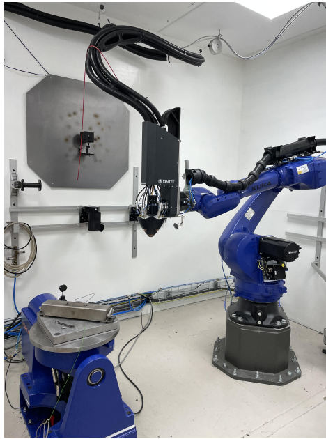
Figure 2.7: The MELTIO system integrated with a KUKA Industrial robot for DED processes at the SINTEF Manufacturing.
