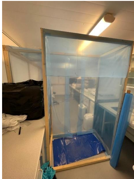
Figure 3.3: Entrance to the laboratory. The laboratory is separated from the surroundings with plastic. The blue sticky mat can be seen at the entrance.
