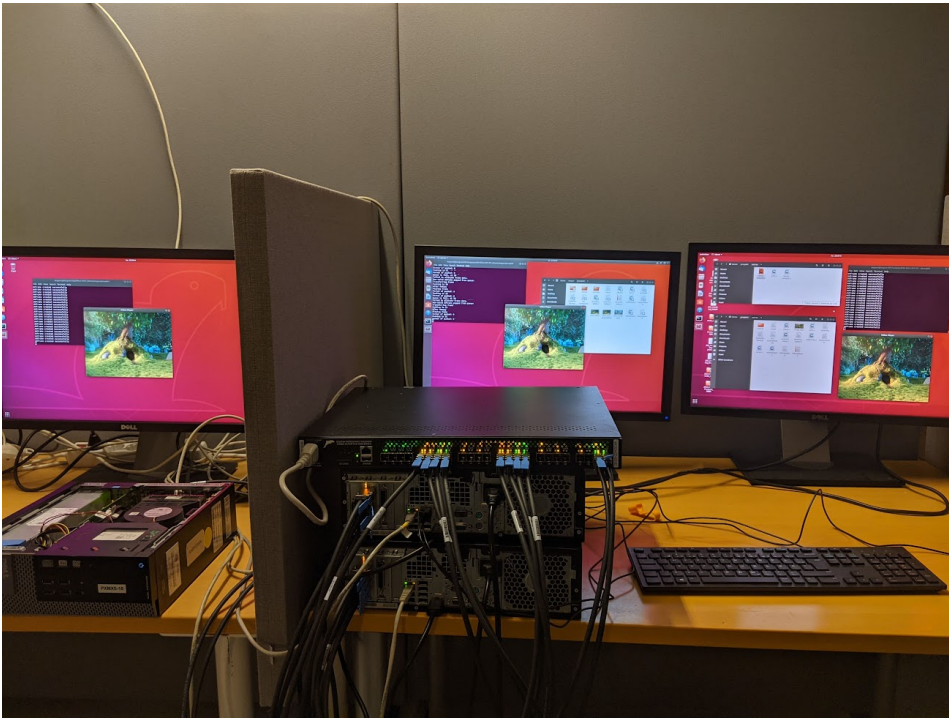
Figure 7.1: Picture showcasing multicast of a video file from one server to two clients. The three nodes are each connected to the PCI-Express switch and a display.
