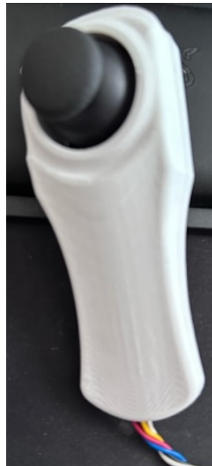
Figure 58: Printed and mounted joystick housing from Thingiverse [65].
