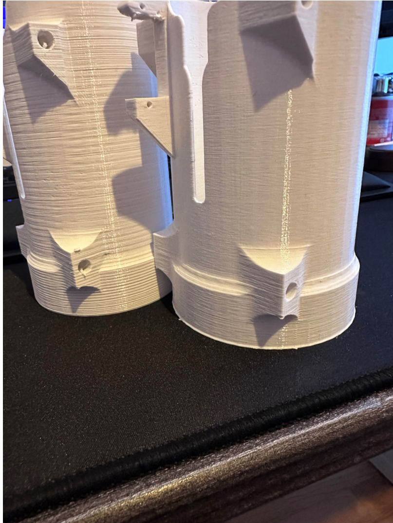
Figure 51: Tube surface roughness.
