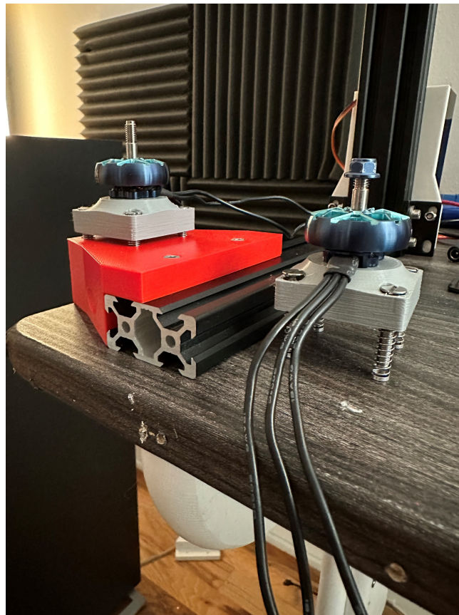
Figure 15: Engine Mount with springs.
