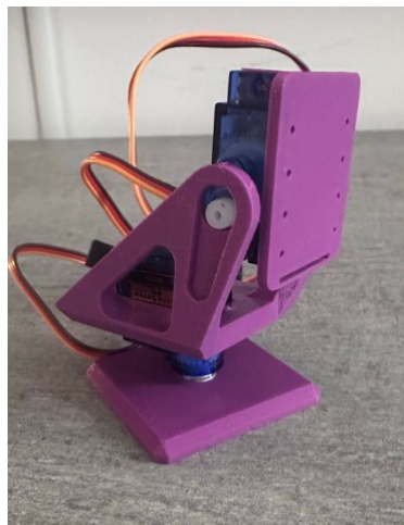
Figure 19: Pan/tilt mechanism from Thingiverse [50].
