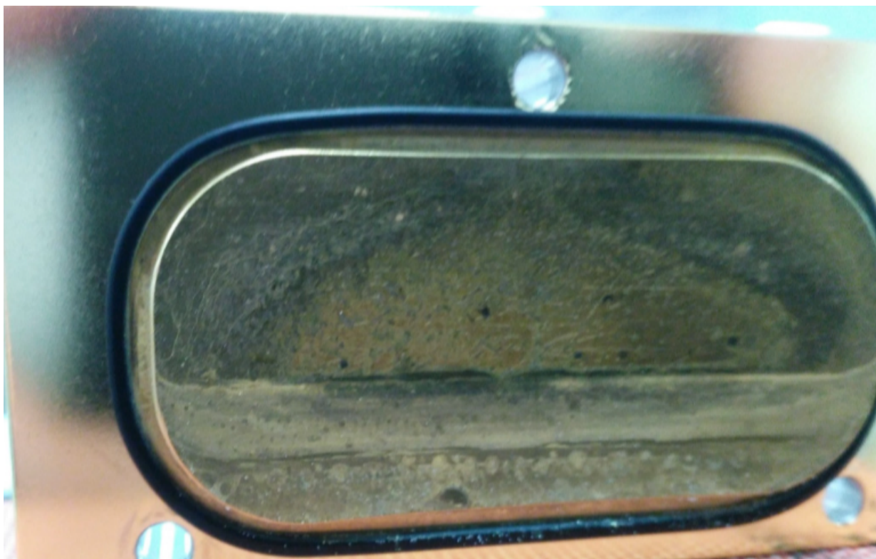
Figure D.2: Contaminated gold plated mirror in the FTIR gas analyzer.
