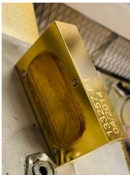
Figure D.3: Contaminated gold plated mirror in the FTIR gas analyzer.
