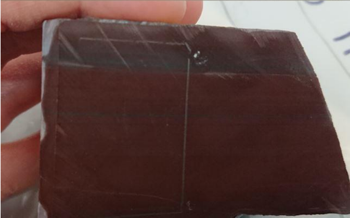
Hand specimens of NYB119256 with the area of the thin section marked.
