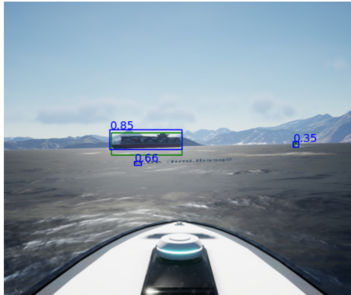
Figure 8.4.: Example of a false positive detection in Experiment 2. A letter in the simulation is detected as a false positive. The green rectangles represent the annotations, the blue rectangles represent the detections, and the blue number is the confidence score.
