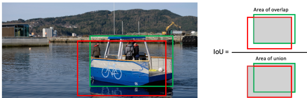
Figure 5.1.: Visualisation of IoU. The green AABB is the ground truth, and the red AABB is the detection. The vessel portrayed in the image is the autonomous ferry milliAmpere, and the image of the vessel is taken from Skoglund (2018).
