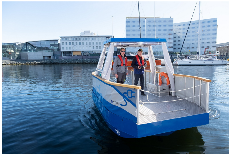
Figure 2.1.: The autonomous ferry milliAmpere developed as part of the Autoferry project at NTNU. In courtesy of Kai Dragland (NTNU (2023)).
