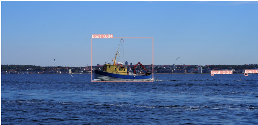
Figure 2.2.: Example of an object detector output, taken from (Schöller, 2022, 18). Each detection comprises an Axis-Aligned Bounding Box (AABB) indicating the spatial extent of the detected object, an assigned object class label, and a confidence score representing the detector’s confidence level in associating the object with that specific class.
