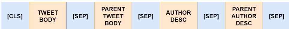
Figure 4.9: Sequence input format for the ContextBERT model with the specialized tokens represented with square brackets.
