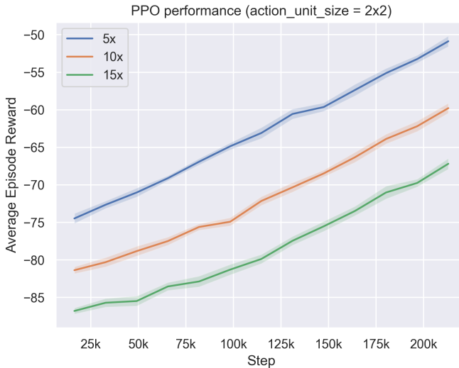
Figure 5.6: The performance of the PPO algorithm (running 8 parallel environments) during training with different action multipliers and with action unit size set to 2 \times 2 . The y-axis shows the average episode reward. The x-axis displays the number of RL environment time steps the algorithm has trained for. The algorithm was trained 20 times for 212 992 time steps in the RL environment for each action multiplier value. The mean of these 20 runs was then plotted, with the shading representing the related 95% confidence interval.
