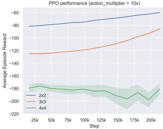
Figure 5.3: The performance of the PPO algorithm (running 8 parallel environments) during training with different action unit sizes and with action multiplier set to 10x. The y-axis shows the average episode reward. The x-axis displays the number of RL environment time steps the algorithm has trained for. The algorithm was trained 20 times for 212 992 time steps in the RL environment for each action unit size. The mean of these 20 runs was then plotted, with the shading representing the related 95% confidence interval.
