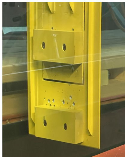
Figure 3.7: Large-drafted models attached with gap distance according to case 3, H/b = 3/11.25 .
