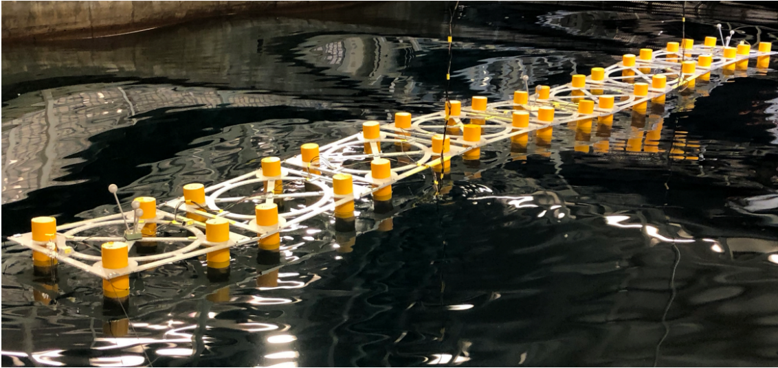
Figure A.5: The model used in Onsrud's Master Thesis. This was an simplified model of the Moss Maritime concept [2], and the scale was 1:20.
