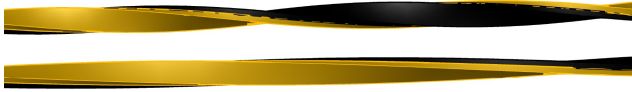
Fig. 1: Two twist pitches, where the top has double the twist pitch of the tape on the bottom.
