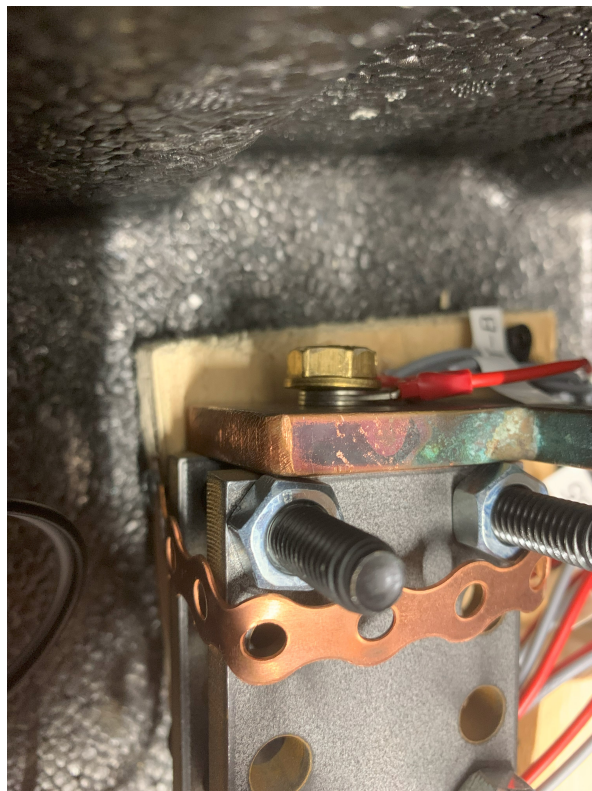
Fig. 30: The placement of the voltage measurement probes meant that an additional resistance through the added copper also was measured for the termination section.
