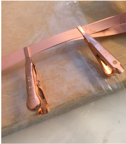
Fig. 20: Two clips were used to keep the already braided HTS tapes in place during the braiding process.
