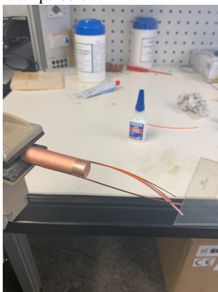
(c) The termination section before it was clamped.
