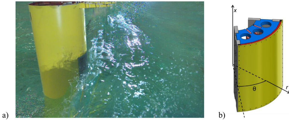
Fig. 1. (a) Wave hitting a monopile during a scaled ocean basin model test at 1:55. (b) A local approximate Froude scaled model shell representing concrete covering a section of the column with a local elastic section.
