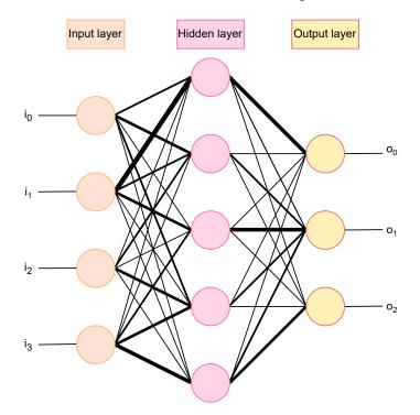
Figure 2.3: A neural network architecture. There are three layer types: one input layer, one or more hidden layers (here: one), and one output layer. There are connections between the nodes in each layer, whose weight is shown through the line's thickness.
