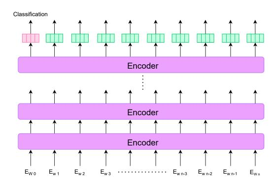
Figure 2.12: The BERT architecture as explained in [17]. The input is embeddings as shown in Figure 2.13. The main part of the BERT model is the 12 or 24 encoder layers that result in a set of output vectors. The first vector (pink) corresponds to the input [CLS] token and is used for classification tasks, while the other (turquoise) vectors are used for token-level tasks.
