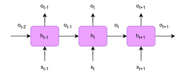
Figure 2.9: Illustration of an RNN where each block corresponds to a time step. The input, output, and the hidden state at time t is given by  $x_t$ ,  $o_t$ , and  $h_t$  respectively.
