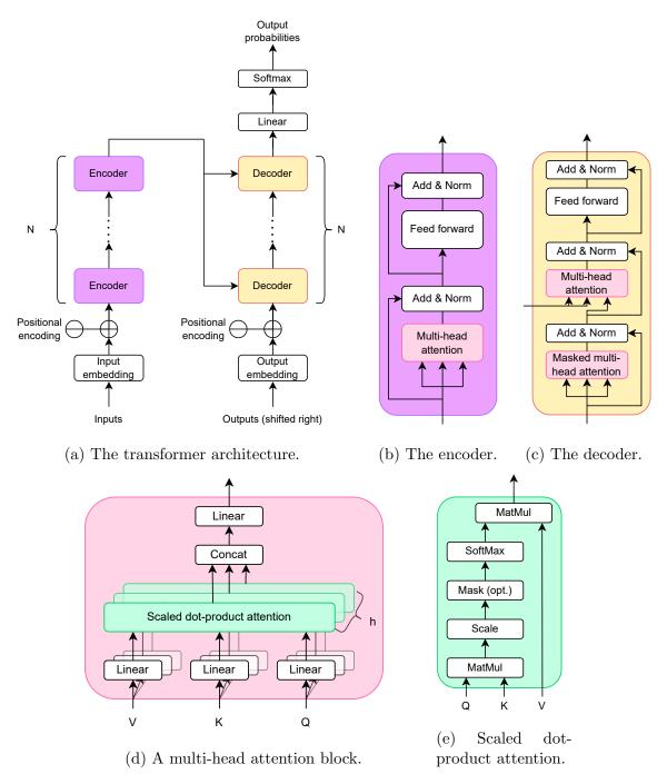
Figure 2.11: The transformer architecture and its parts as presented in [64].
