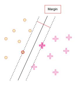
Figure 2.4: An illustration of how an SVM solves a binary classification task. The two points with a thicker edge are support vectors that limit the size of the margin.
