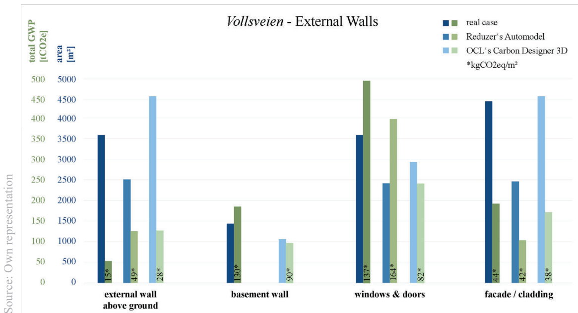
Figure 22 Comparison of the amount and GWP of sub-elements of the external wall category between real case and predictions for Case Study 1
