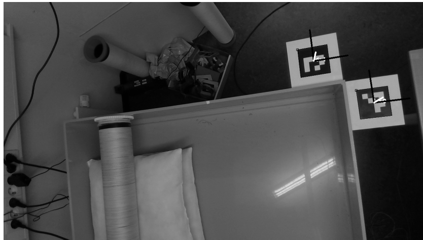
(b) Intel RealSense image of incubator with new marker positions and their frames visualized
