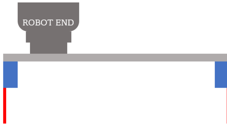
Figure 7.3.: An asymmetric gripper mount of the gripper could increase the reach of the robot, but torque would be introduced due to the center of mass being shifted.
