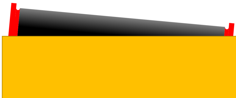
Figure 6.10.: Illustration of a tube not laying horizontally in the incubator seen from the short side
