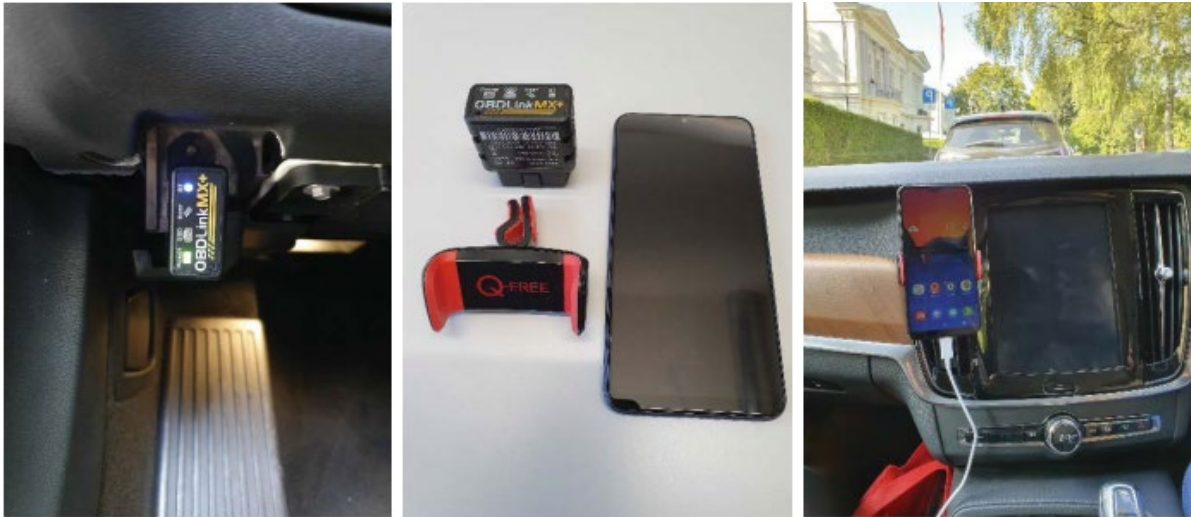
Figure 11 Equipment used for GeoSUM pilot project (left: Dongle, middle: all equipments, right: smartphone setup). (GeoSUM project report, figure 26, p. 47).
