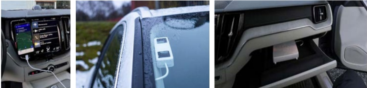
Figure 14 Equipment used for GeoFlow pilot project (left: smartphone setup, middle: antenna, right: processing unit). (Source: GeoFlow project report, figure 1, p. 6).
