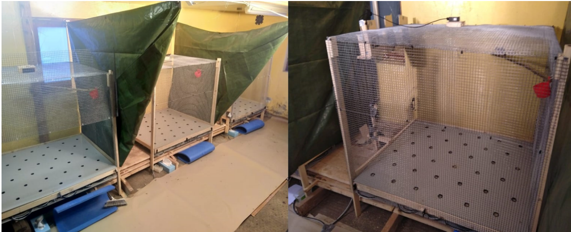
Figure 2.1: Experimental set-up with 'checkerboard' feeders. The feeder plates are 1x1.2 meters, with 36 evenly spaced wells.
