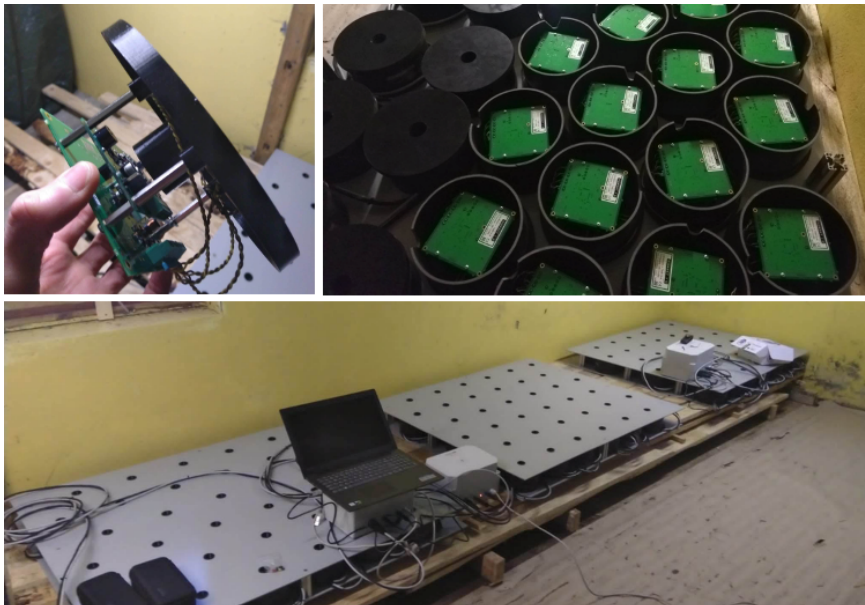
Figure 2.2: The RFID-antennae that are connected to each well. All antennae are compatible with the PIT-tags attached to the leg rings of all individuals.
