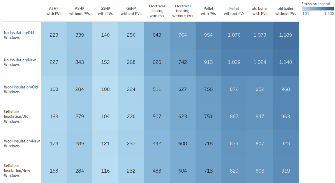
Figure B.8: Emission (KgCO 2 eq/m 2 ) of semi-detached house, built in 1990 to 2000 through 60 years, Berlin weather
