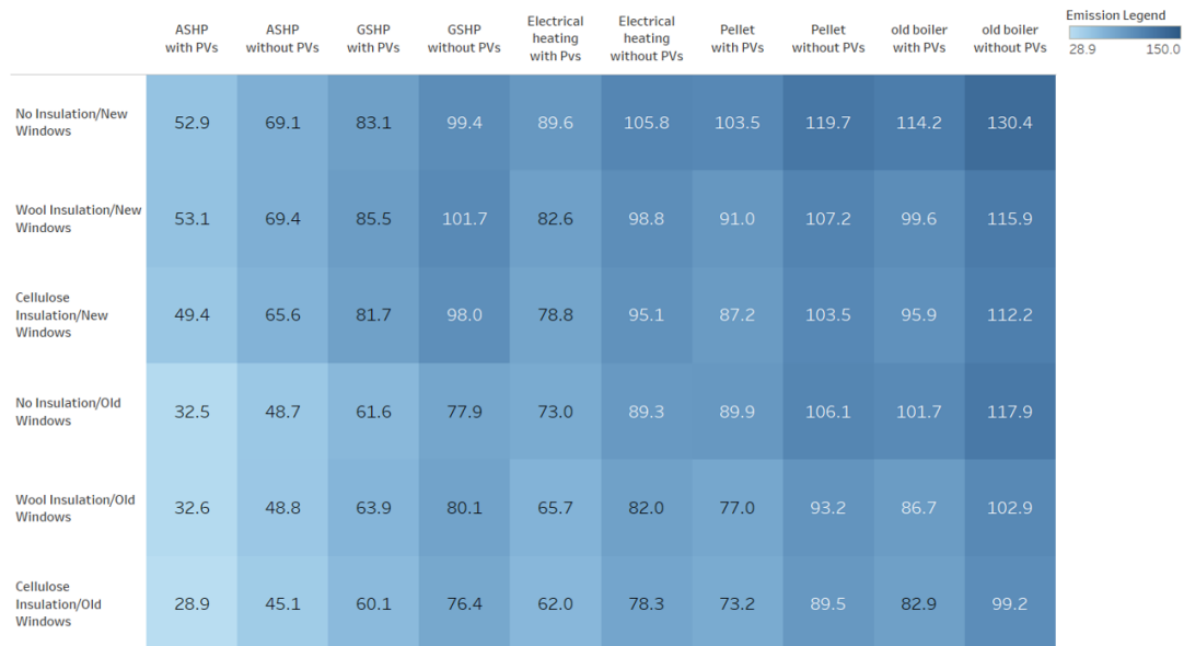
Figure C.3: Emission (KgCO 2 eq/m 2 ) of detached house, built in 1980 to 1990 through 60 years, 2050 weather data
