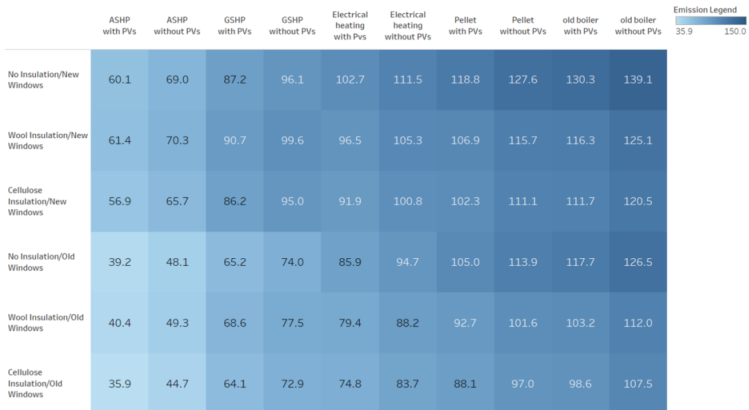
Figure C.7: Emission (KgCO 2 eq/m 2 ) of semi-detached house, built in 1980 to 1990 through 60 years, 2050 weather data
