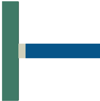
Figure 4.3: The three initial parts, and their location in the assembly. Green is column, blue is regular beam and grey is connection zone.
