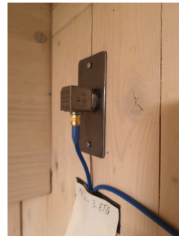
(b) Accelerometer attachment
