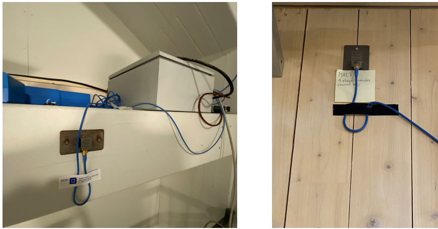
(a) Accelerometer mounting on a glulam beam (b) Accelerometer mounting on a CLT plate
