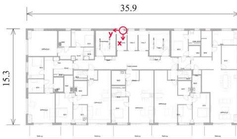
(b) Building frame view with accelerometer positions
