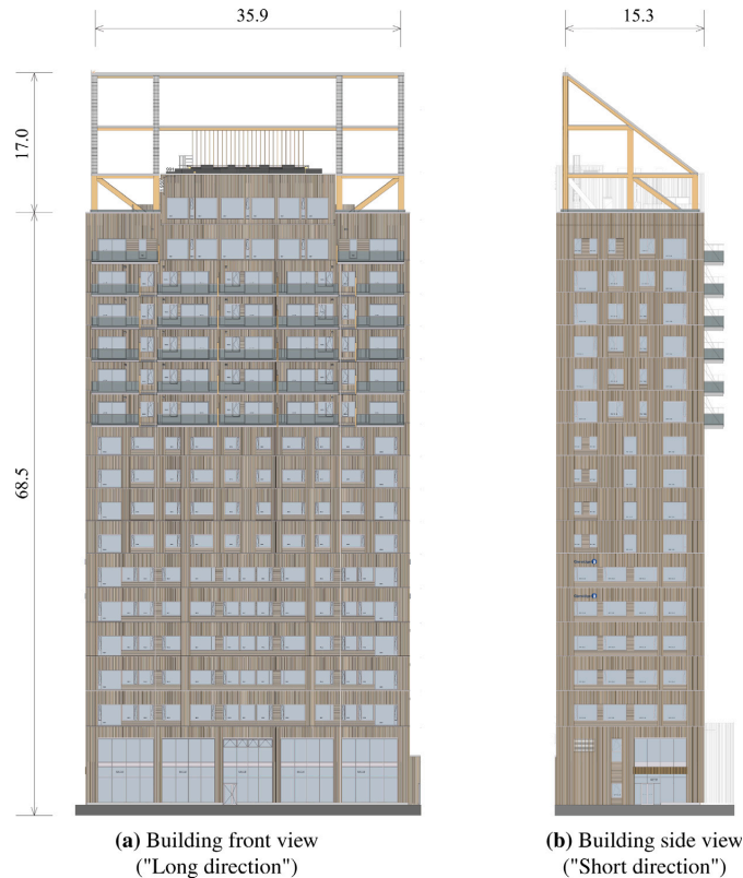
Fig. 1. Mjöstärnet building (dimensions in m).
