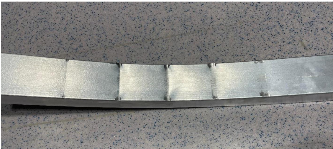
Figure 7: Specimen bent using the steel axles (Lundby, 2023).
