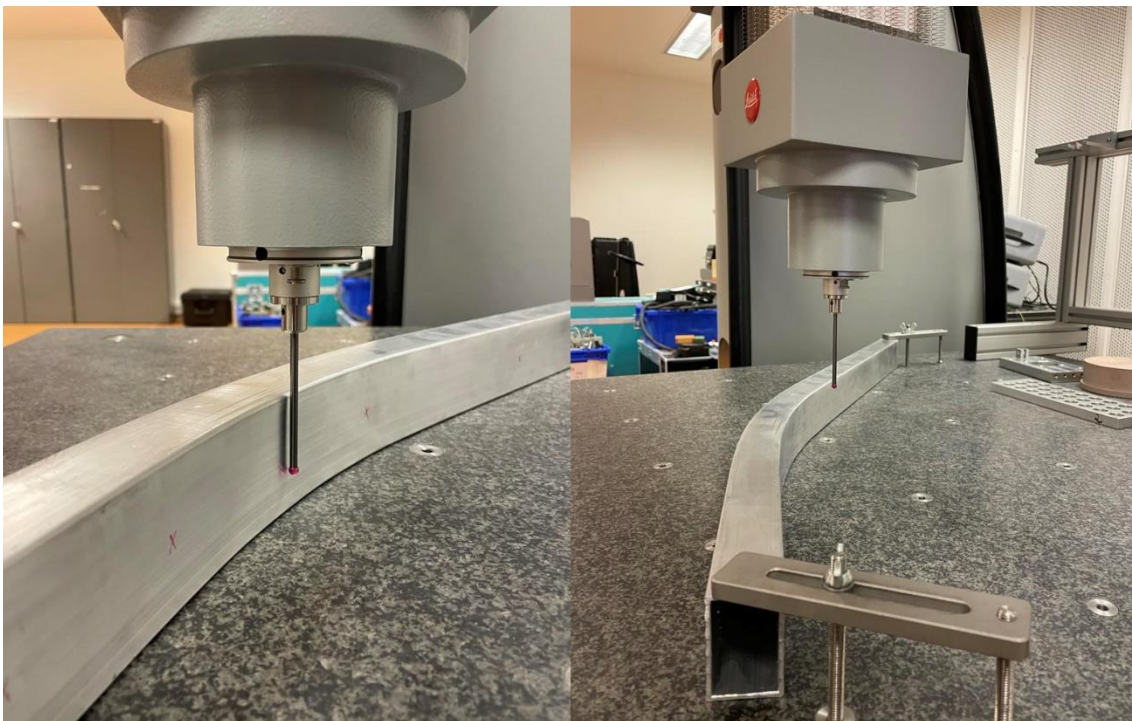
Figure 35: Measuring the specimen along the marked coordinates. The left picture showcases the mapping of the curvature, while the right highlights the mapping of the straight parts.
