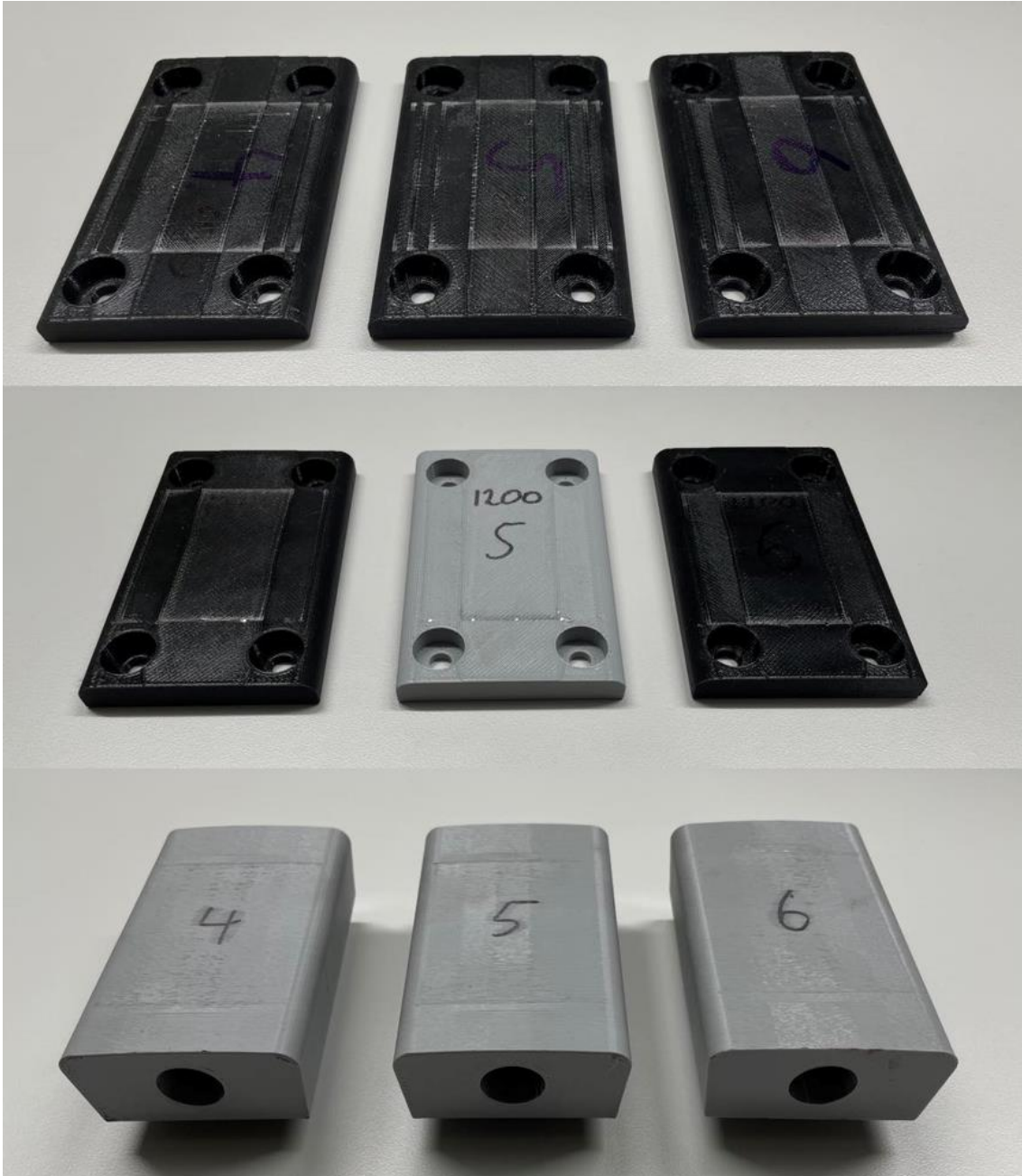
Figure 40: Upper part of the AM tool number 4, 5, and 6 of the new R600 AM tools (top), the new R1200 AM tools (middle), and tool number 4, 5, and 6 of the tools from iteration 2.
