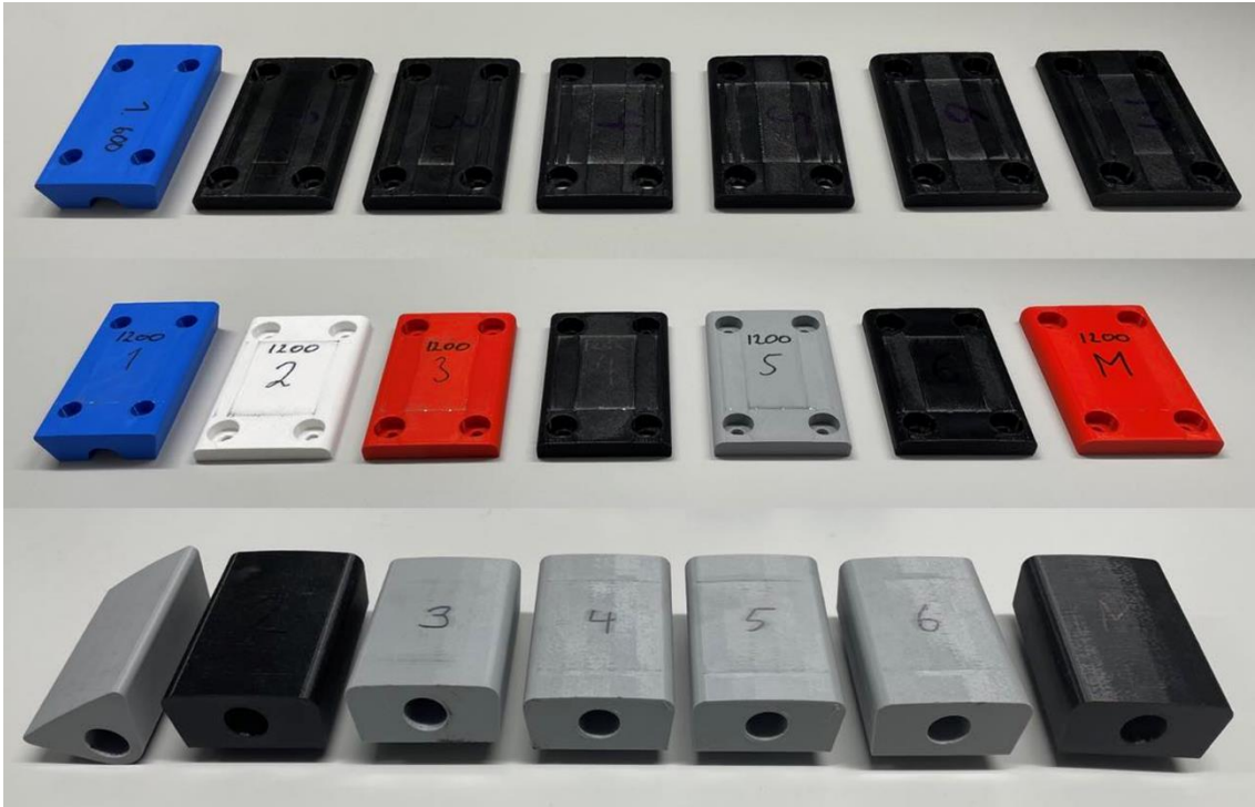
Figure 39: The AM tools after the completion of the bending experiments. The tools on the top are the upper parts with a R600 curvature, the tools in the middle are the upper parts with a R1200 curvature, while the tool on the bottom are the tools from the second iteration of the AM tools.
