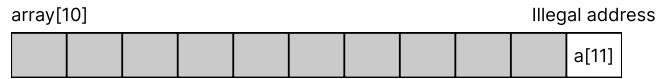
Figure 2.6: Memory layout of an array of 10. Gray elements represent addresses that are allocated to the array, and the white element at the end represents a memory address outside the allocated memory space
