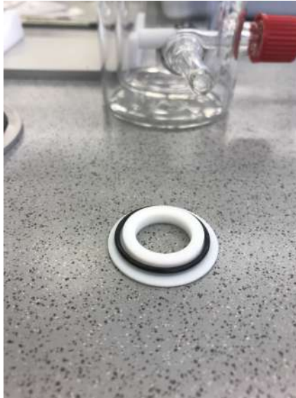
Figure 3.8: The teflon fitting which was prone to leakages during the B240 and B280 experiments. It was positioned between the sample holder and the cell chambers, see figure 3.7.
