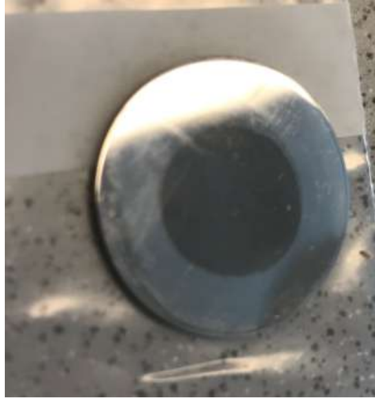
Figure 3.6: The Pd coating made a visible deposit on the samples.
