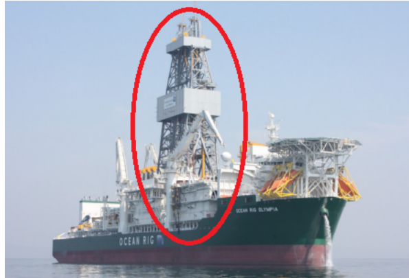
Figure 17: Derrick from Ocean Rig Olympia [61]
