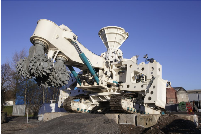
Figure 6: Auxiliary cutter built by Soil Machine Dynamics, owned by Nautilus Minerals [44]
