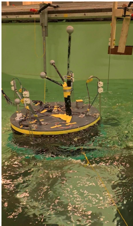
(d) Configuration 3 during wave overtopping
