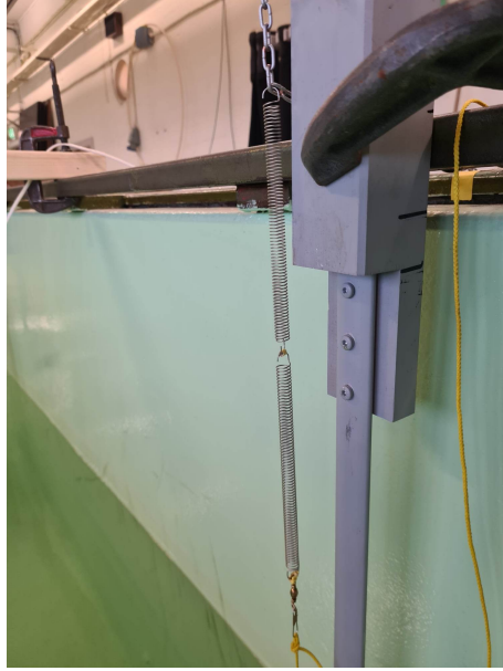
Figure 12: Close up of the connection between the springs. Two 50 N/m springs in series creating a 25 N/m spring.
