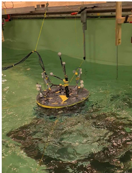
(c) Configuration 3 during wave overtopping
