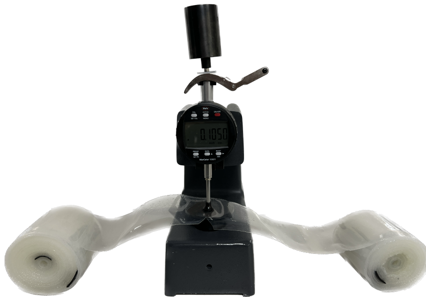
Figure 3.9: Micrometer used for thickness measurements.
