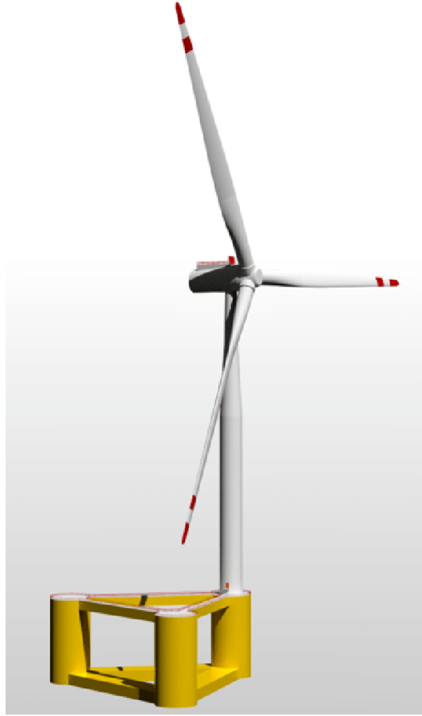
Figure 4.2: INO WINDMOOR design (Souza et al., 2021)
