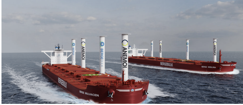
Figure 3.4: Berge Mulhacen and Berge Neblina with Anemoi rotor sails [7]
