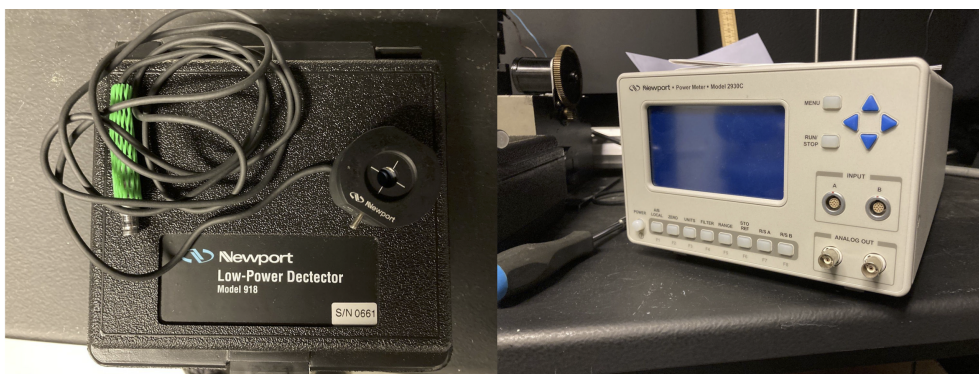
Figure 5.5: To the left a Newport 918 low power detector and to the left a Newport 2930C dual channel optical power meter.
