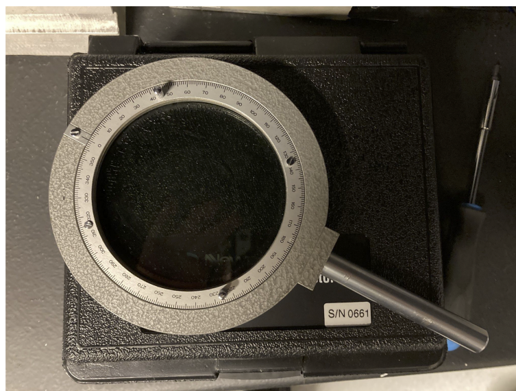
Figure 2.7: Manual rotational filter used with an attached thin film polarizer to calibrate the motorized filter wheel.
