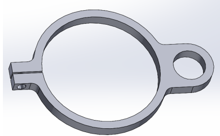
Figure 5.14: Machined line guider for securing the vehicle during testing in the sea
