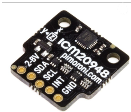
Figure 5.7: ICM20948 motion sensor mounted on the PIM448 module, reproduced from [17]
