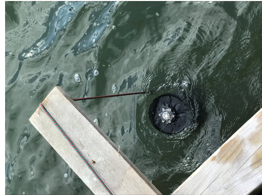
(b) The safety line in set up at a distance from the dock, to prevent the BV from colliding with the dock wall during the mission.
