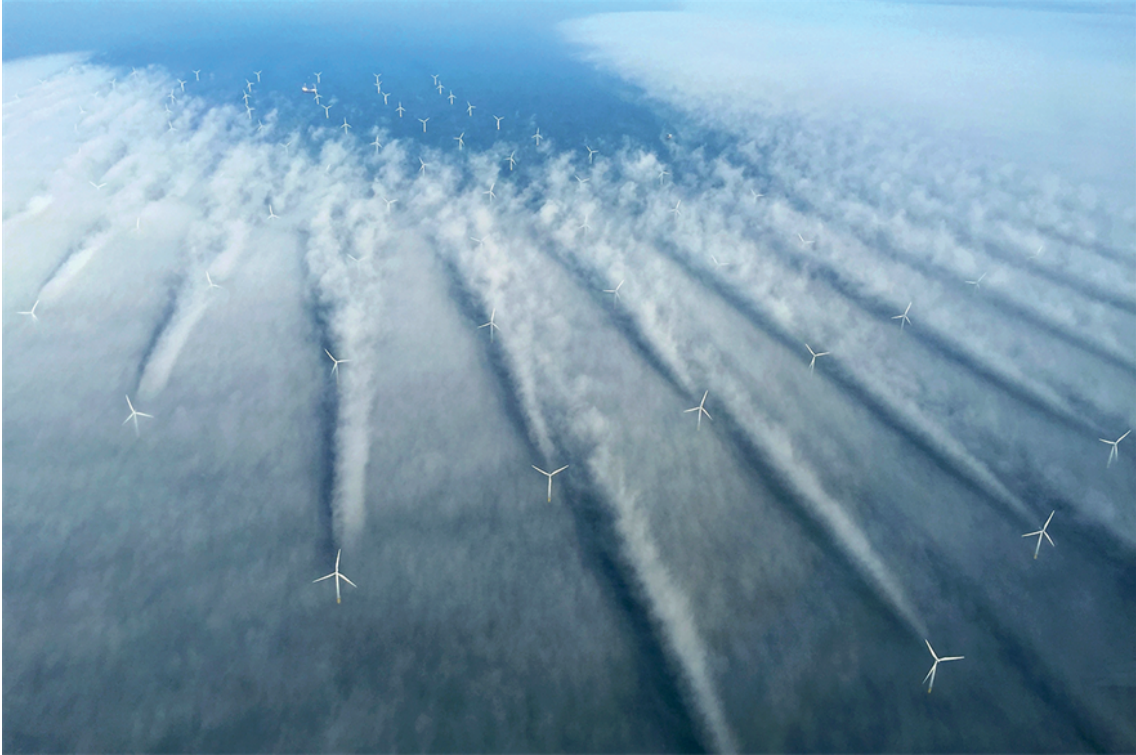
Figure 3.5.1: Visualisation of the turbine wake effect [43]
