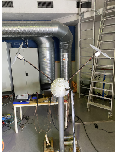
FIGURE 5.7: Static load test in parallel configuration
