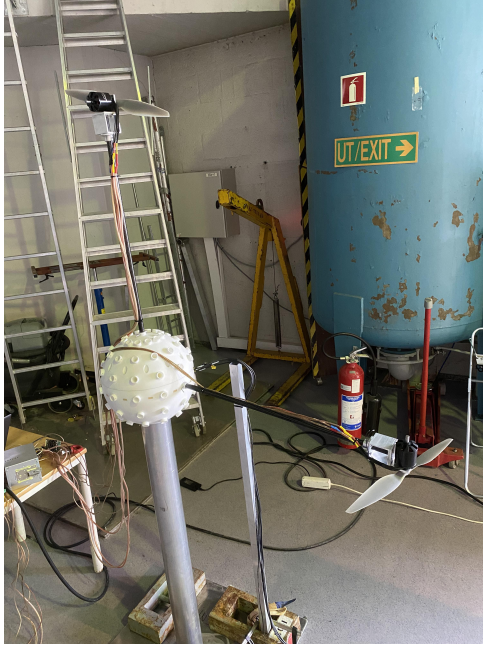
(A) The setup for thrust curves in F_x and F_z
