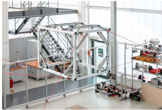
FIGURE 2.1: Setup of CDPR - from [10]
