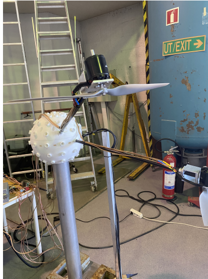
FIGURE 5.14: Configuration of the static rotor 22.5° behind and 30° to the side of the dynamic rotor
