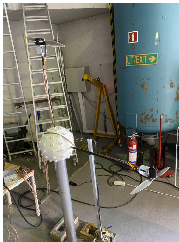
FIGURE 5.17: Configuration of perpendicular interaction test with 90^\circ angle between the rotors
