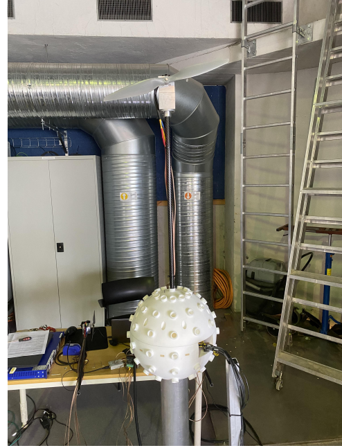
(B) The setup for thrust curves in F_y
