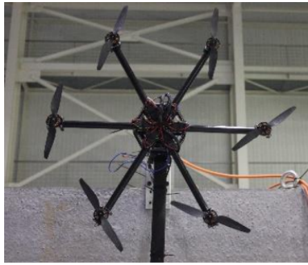
FIGURE 2.5: Multi-fan setup with 6 rotors - from [12]
