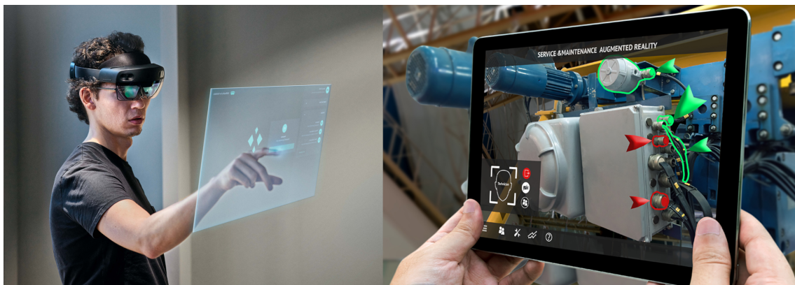
Figure 8.2: Example of See-through AR (left) and Monitor-based AR (right).
