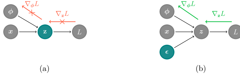
Figure 3.3: The reparameterization technique shown in a simplified computation graph. The figure is inspired by Kingma and Welling (2019). (a) The stochastic vector \mathbf{z} blocks the loss gradient from reaching \phi . (b) Extracting the stochastic component \epsilon from \mathbf{z} permits gradient flow.
