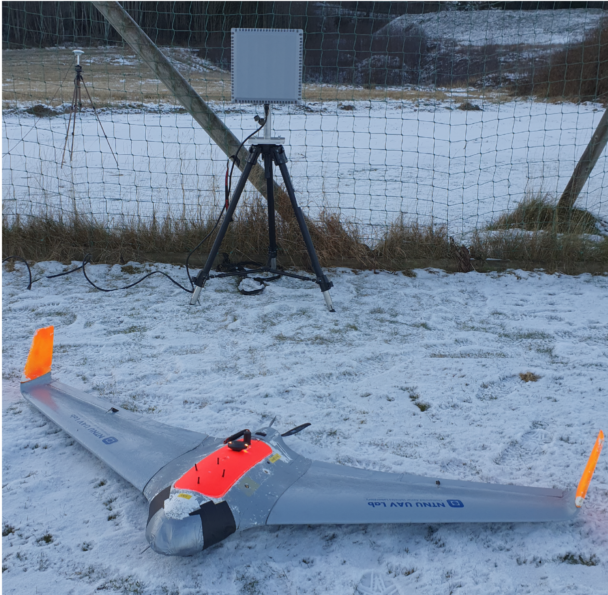
Figure 5.2: Image of the Skywalker X8 UAV and a CRE189 ground unit. Taken from [22].
