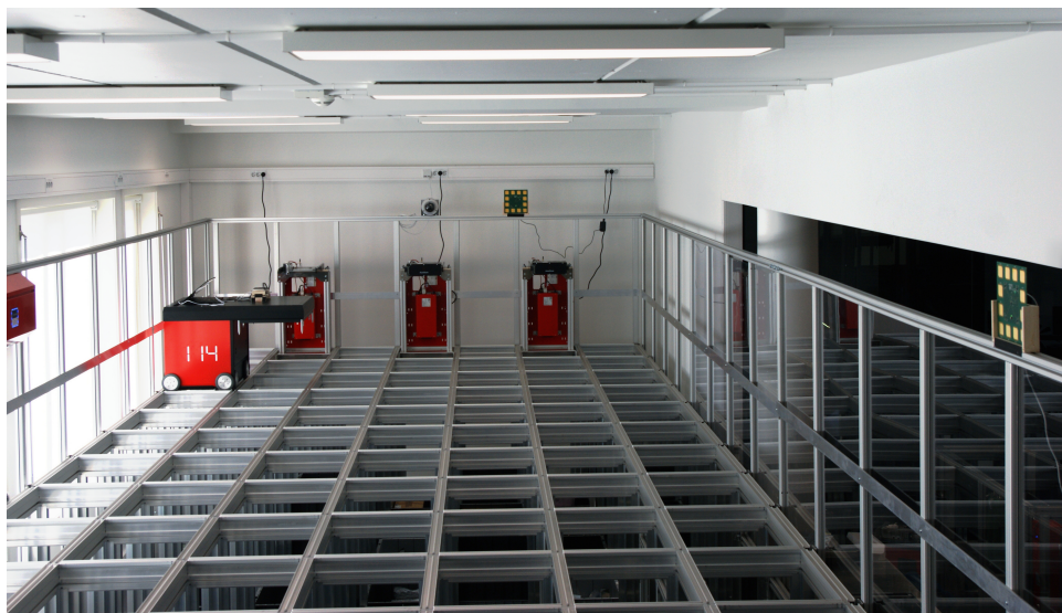
Figure 4.1: Robot with antenna receiver. The robot is currently on cell (39, 8) and array F is visible on the far end and array D is visible on the right hand side. Note that we use gripper-centric coordinates which is where the receiver is placed, the body of the robot is on cell (40, 8)
