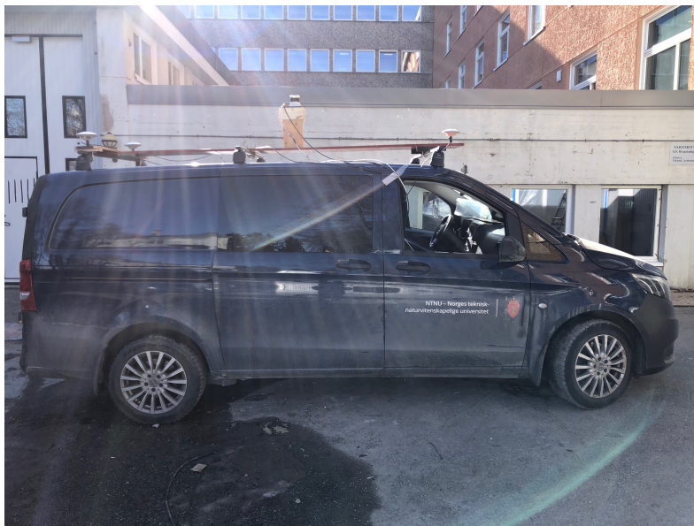
Figure 4.5: Photograph of the Mercedes Vito car with sensors installed on the roof. The sensors are mounted on a sturdy platform, with two GNSS antennas positioned at the rear, one at the front, and the LiDAR-IMU platform elevated in the center.
